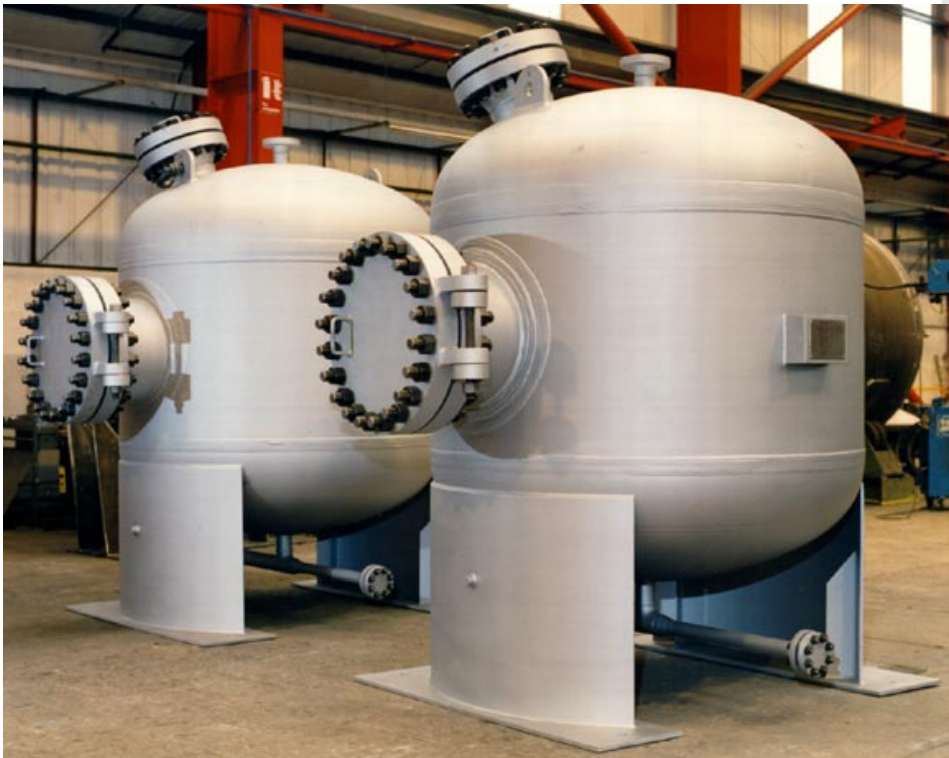
2 No LLAC-3400-030 Series 600 Lean Amine Activated Carbon Filters Design Code BS5500 Cat.1, Wall Thickness - 75mm Supplied to Chiyoda - Foster Wheeler for OMAN LNG
